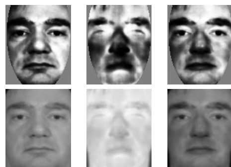
Fig. 6. Examples of image fusion. Rows differs from the preprocessing that has been applied. Left:Visible, Center:Infrared, Right: Fusion.
