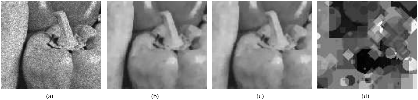
Fig. 2. (a) Noisy input image damaged by gamma noise (PSNR=21.14). (b) Denoised image using the GLR after variance stabilization (PSNR=27.42). (c) Denoised image using the GLR adapted to gamma noise (PSNR=27.53). (d) Image composed of the atoms of the dictionary.
