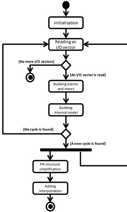
Figure 2. Stages of the identification algorithm
