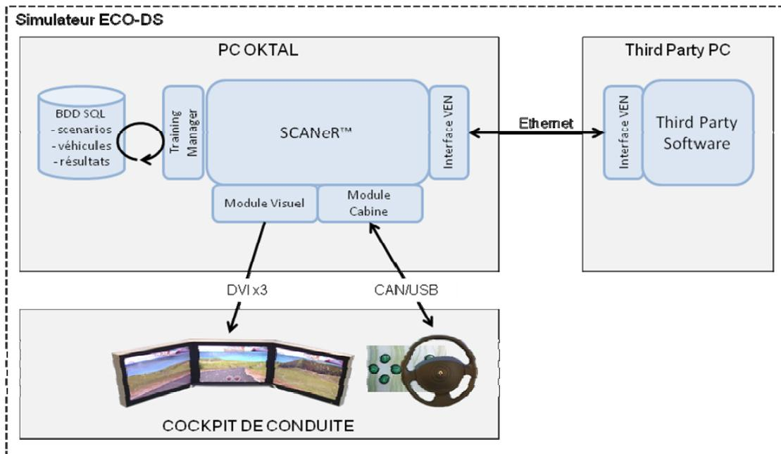
Figure 2: ECO-DS simulation architecture
