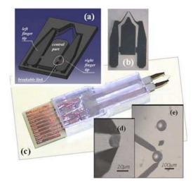
Fig. 6 Silicon finger-tip (10 µm thick)
