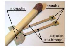
Fig. 3 Piezoelectric actuators of the FEMTO-ST microgripper
