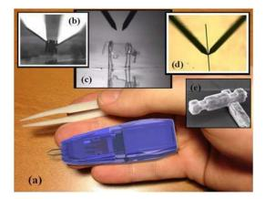
Fig. 7 a PiTweez from PERCIPIO-ROBOTICS, **b** micromanipulation of a silicon micro part 40  $\mu$ m × 40  $\mu$ m × 5  $\mu$ m, **c** polymer microcow to demonstrate micro-assembly (500  $\mu$ m long, smallest nose part is 50  $\mu$ m × 50  $\mu$ m × 5  $\mu$ m), **d** fiber, 7  $\mu$ m diameter, **e** silicon parts assembly, 7  $\mu$ m width
