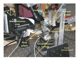
Fig. 25 Micro-assembly cell comprising one 4 DOF piezoelectric microgripper, two robotized arms split onto 9 DOF (micropositionner and nanopositionner), one vacuum gripper and two high magnification cameras
