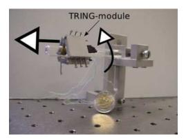
Fig. 9 A photography of the TRING-module stick-slip microrobot
