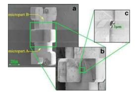
Fig. 21 Some images of the assembled structure from a scanning electron microscope
