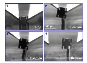
Fig. 33 Insertion assembly
