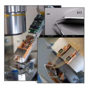
Fig. 8 a PiezoTweeze prototype, b and c details of polymer finger-tips
