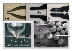
Fig. 5 Nickel finger-tips (200 µm thick)
