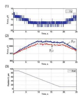
Fig. 24 Forces acting during a guiding task: (2) measured contact forces between micro-object and fingers 1 and 2 (I) is the estimated contact force between micro-object and rail and (3) is the positioning of the micro-object along the rail
