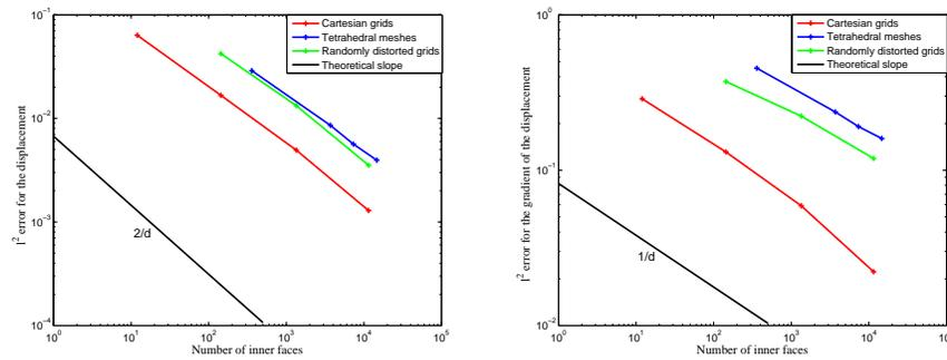
**Fig. 2**  $l^2$  error for the displacement and for the gradient of the displacement function of the number of inner faces for the Cartesian grids, the randomly distorted grids and the tetrahedral meshes.
