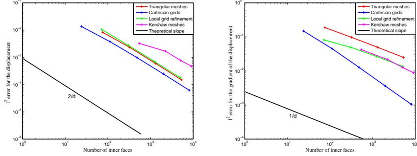
**Fig. 1**  $l^2$  error for the displacement and for the gradient of the displacement function of the number of inner faces for the triangular meshes, the Cartesian grids, the local grid refinement and the Kershaw meshes.
