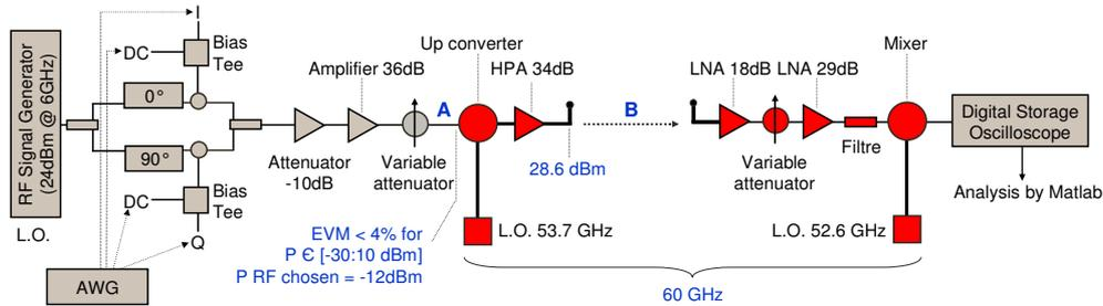
Figure 2 : Experimental setup for the mm-wave radio link.
