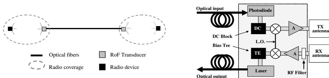
Figure 1 : RoF tunnel at the left (point-to-point link) and RoF transducers at the right.
