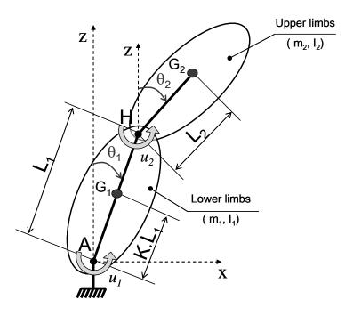
Fig. 1: Double inverted pendulum model of human standing.
