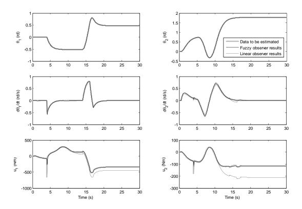
Fig. 3: Angular position and torques estimations following a complex trajectories simulation.
