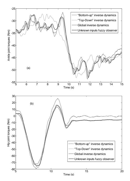
Fig. 9: Comparison of inverse dynamics approaches and the fuzzy unknown inputs observer for the CTE experiment, (a) ankle torques estimations, (b) hip torques estimations
