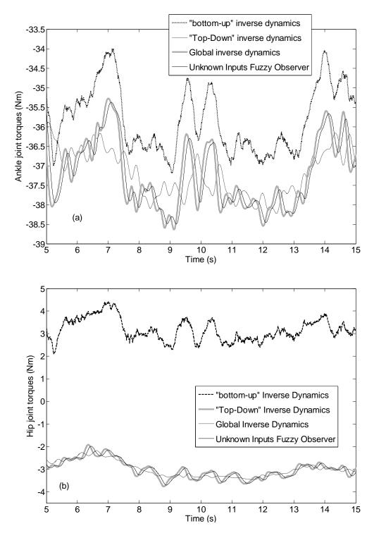
Fig. 11: Comparison of inverse dynamics approaches and the fuzzy unknown inputs observer for the QS experiment, (a) ankle torques estimations, (b) hip torques estimations
