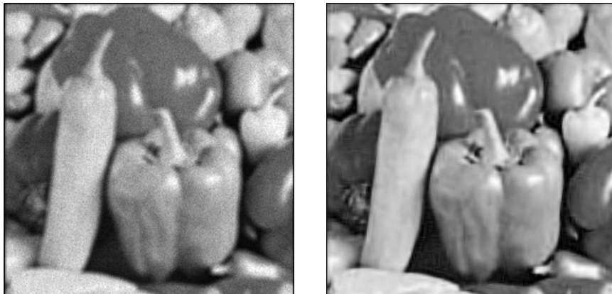
Figure 1: Deblurring: Degraded image, SNR=19.3 dB (left) and restored image (right) with the proposed algorithm, SNR=24.3 dB.
