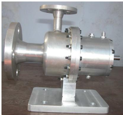
**Fig. 5.** A high-speed micro turbine for Organic Rankine cycle
