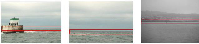
Fig. 6: Limiting the image analysis area by inertial unit.
