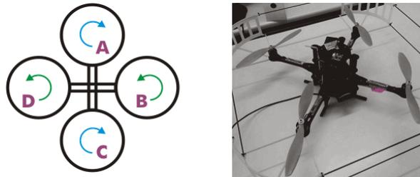
FIG. 1.1. *The quadrotor(right) from Ascending technologies(Available at ESIEE).*
