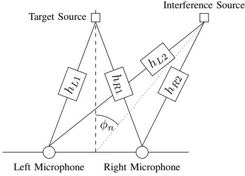
Fig. 1: Example scenario, where the variations of  $h$  are impulse responses representing the room. The signal detected at each microphone is a convolutive mixture of each source. The dashed line indicates the imaginary line where, at all positions, the target source is equidistant to both microphones.  $\phi_n$  denotes the angle of the interference source.
