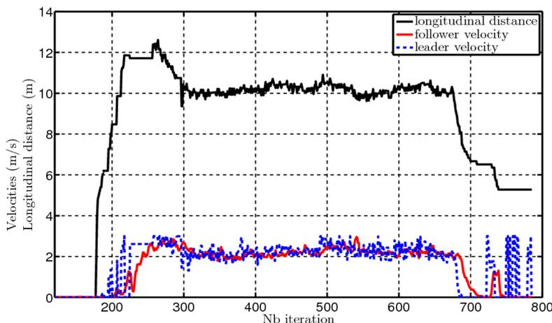
Figure 8: Longitudinal distance and velocity of robots
