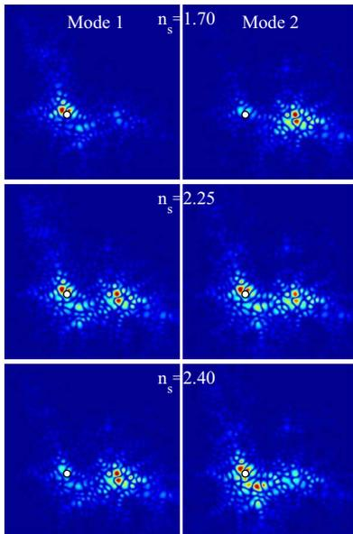
Fig. 2. (Color online) Spatial distribution of the field amplitude for Mode<sub>1</sub> and Mode<sub>2</sub> of Fig. 1 for three different values of the refractive index of the scatterer located at the white spot. Media 1 displays the evolution of the mode profiles as  $n_s$  increases from 1.05 to 2.40.
