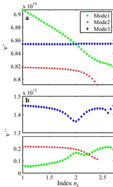
Fig. 1. (Color online) Monitoring of a. the real part  $\nu'$  and b. the imaginary part  $\nu''$  of three localized states as the refractive index,  $n_s$ , of a particular scatterer (shown in Fig. 2) is varied from 1.05 to 2.70. The Y axis has been split in b to span a broad interval of  $\nu''$ .
