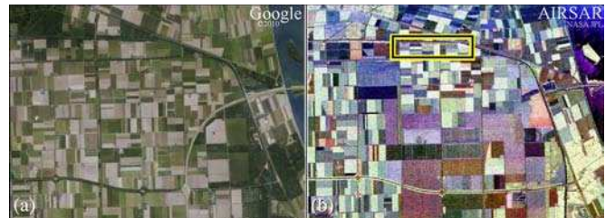
Fig. 3. Flevoland, The Netherlands. (a) Google Earth image of the area. (b) Pauli RGB image of the NASA/JPL AirSAR fully polarimetric data set (Red, |S_{HH} - S_{VV}| ; Green, |S_{HV} + S_{VH}| ; Blue, |S_{HH} + S_{VV}| ). The outlined area in (b) is a test area in which a number of high-voltage transmission towers are present. The original image has a size of 1024 \times 750 pixels.
