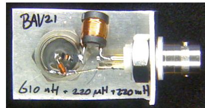
Figure 9. Diode mount with the diode soldered directly to a BNC connector. A series network of inductors is connecting the diode to the voltmeter.
