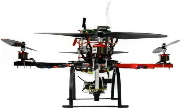
Fig. 1: The four-rotor aircraft experimental platform.
