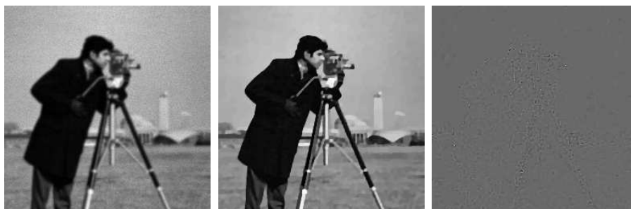
Fig. 3. Result for the 'cameraman' image B1 1200 corresponding to Table 3. Corrupted image (left), restoration result by the Anscombe constrained model and Alg. 1 (middle), difference image between the middle image and the one recovered by I -divergence constrained model and Alg. 2 (right). The gray values in the difference image are between -10 and 10, while the image values were scaled up to 1200.
