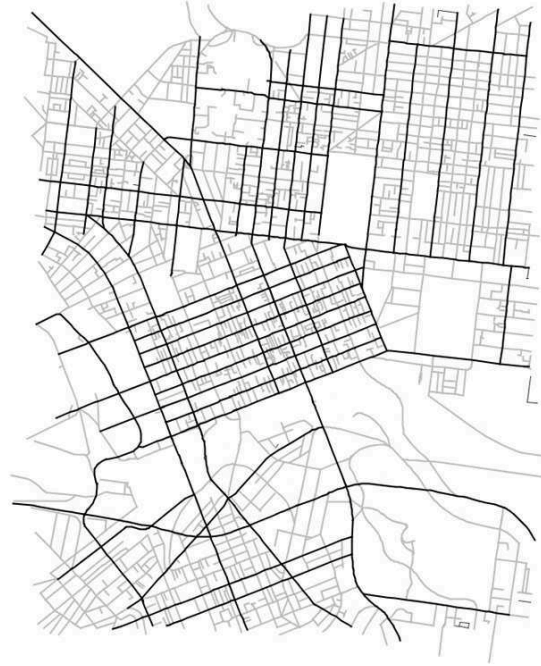
Fig. 7. Street network representations of streets of inner suburbs of Melbourne, with prominent streets highlighted (52 streets with fast choice values \sigma above mean).
