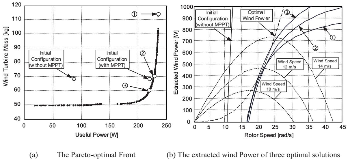
**Fig. 3 : Pareto-optimal configurations compared with a non-optimized wind turbine**
