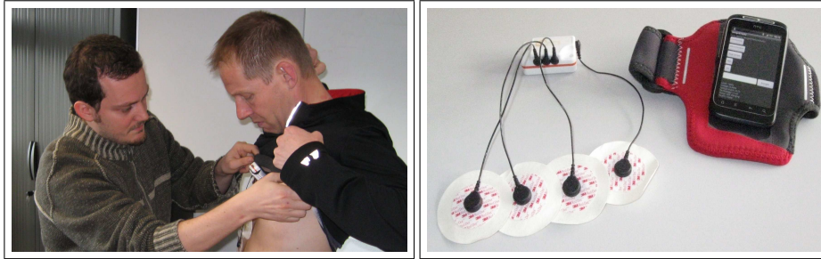
Fig. 1. A volunteer is equipped with an ECG-enabled SHIMMER sensor and a smartphone (which can be worn in an armband or in a pocket)
