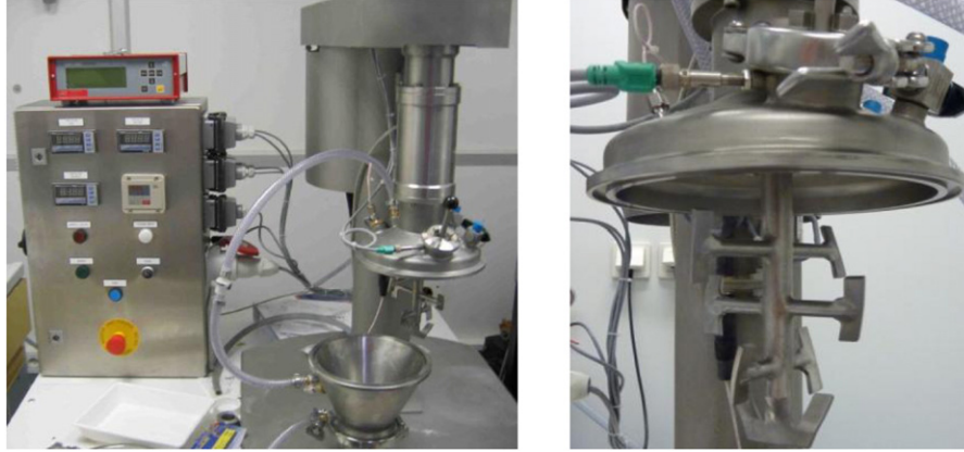
Fig. 3. Schematic diagram of the high shear mixer "Cyclomix".
