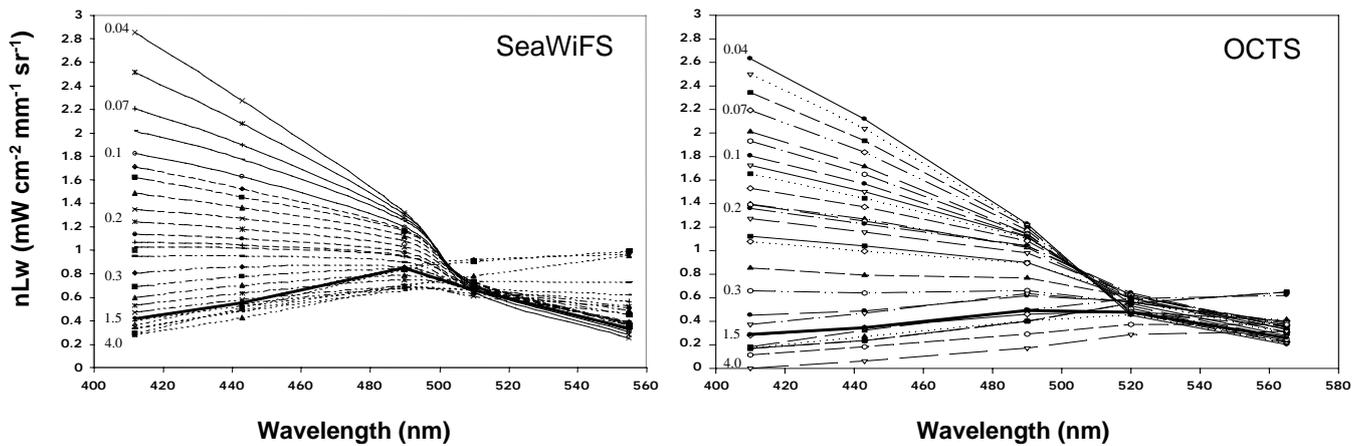
**Fig. 1.** A comparison between the SeaWiFS (left) and OCTS (right) reference model ( $nLw_{ref}$ ) of the normalized water-leaving radiance ( $nLw$ ) as a function of wavelength for various chlorophyll-*a* concentrations ( $Chl-a$ ).
