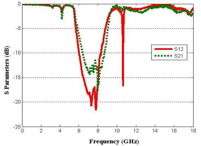
**Fig. 6.** Experimental results on bulk ferrite substrate ( $1000\ \mu m$  thick) prototype
