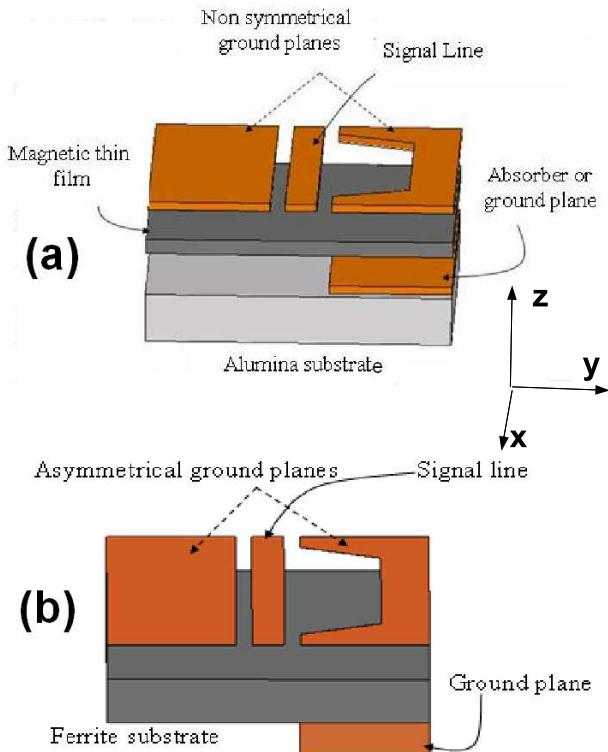
**Fig. 2.** Coplanar isolator structure (a) YIG layer on alumina substrate, (b) only YIG substrate
