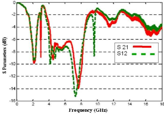
**Fig. 7.** Experimental results on ferrite layer ( $150 \mu m$  thick) prototype
