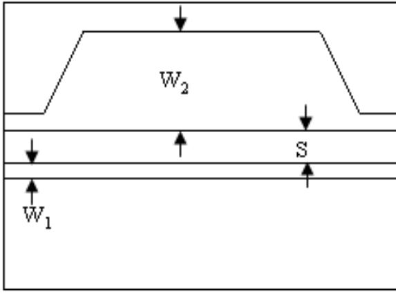
**Fig. 3.** Coplanar isolator structure: top view and dimensions
