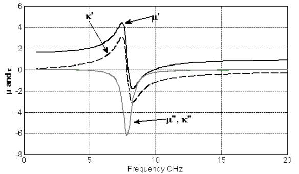
**Fig. 1.** Ferromagnetic resonance: real and imaginary parts of the elements of the permeability tensor versus frequency (223 kA/m applied field).
