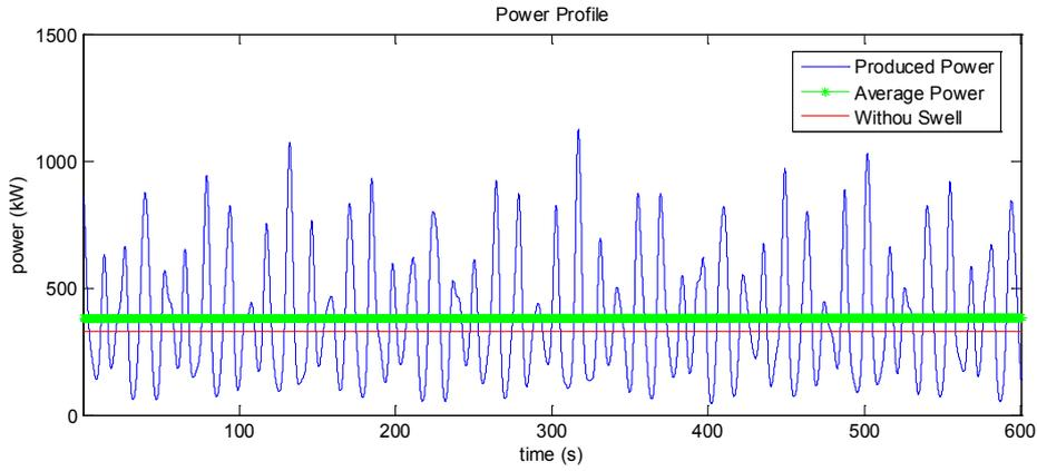
Fig. 6. Power profile of a marine current turbine.
