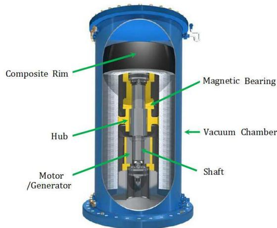
Fig. 10. Typical flywheel energy storage system [15].
