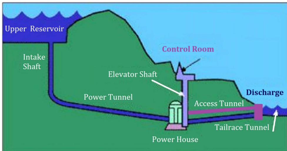
Fig. 13. Schematic of Pumped Hydro Storage plant [34].
