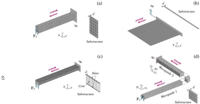
Figure 1: Illustration of several elastic waveguides and representative substructures: (a) beam-like structure; (b) plate; (c) sandwich structure; (d) coupled beam-like structures.
