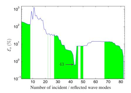
Figure 7: Error bound  $\mathcal{E}_s$  as a function of the number m of incident / reflected wave modes for a Reissner-Mindlin plate with one edge subjected to a prescribed transverse displacement. (Green shaded area): case where assumptions  $||\widetilde{\mathbf{A}}^s|| \leq ||\mathbf{A}^s||$  and  $||\widetilde{\mathbf{A}}^{\star s}|| \leq ||\mathbf{A}^{\star s}||$  are satisfied.
