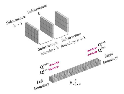
Figure 2: Representation of substructure boundaries (their number is N+1 along the waveguide) and representation of the conventions made to describe the incident / reflected waves at the left and right boundaries of waveguides.
