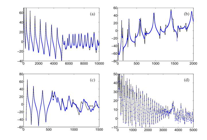
Figure 3: Frequency response function (quadratic velocity (dB)) for beam-like structure (a), plate (b), sandwich structure (c), coupled system (d): (——) FE reference solution; ( $\bullet \bullet \bullet$ ) WFE solutions when the wave modes are selected by the classic procedure (number of retained wave modes: m = 30 (a), m = 60 (b), m = 80 (c) and m = 30 (d)).
