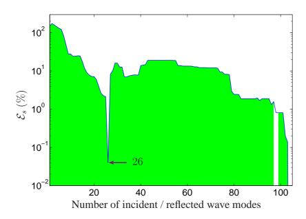
Figure 4: Error bound  $\mathcal{E}_s$  as a function of the number m of incident / reflected wave modes for a clamped beam-like structure whose left end is subjected to a uniform transverse force field. (Green shaded area): case where assumptions  $||\widetilde{\mathbf{A}}^s|| \leq ||\mathbf{A}^s||$  and  $||\widetilde{\mathbf{A}}^{\star s}|| \leq ||\mathbf{A}^{\star s}||$  are satisfied.
