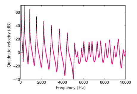
Figure 5: Frequency response function of a clamped beam-like structure whose left end is subjected to a uniform transverse force field: (——) FE reference solution; (•••) WFE solution with m=26 wave modes selected by means of the error bound  $\mathcal{E}_s$ .
