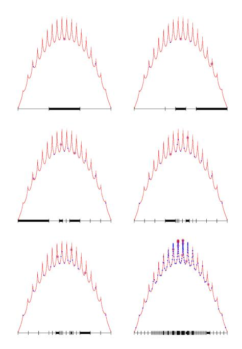
**Figure 4.4:** The first 5 iterations of the SOO algorithm and the resulting tree  $\mathcal{T}_n$  after n = 150 function evaluations for the garland function  $f(x) = x(1-x)(4 - \sqrt{|\sin(60x)|})$ .
