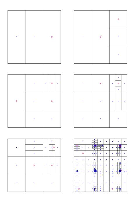
**Figure 4.6:** The first 5 iterations of the SOO algorithm and the resulting tree  $\mathcal{T}_n$  after n = 150 function evaluations. Here we considered the 2-dimensional function  $f(x_1, x_2) = f(x_1)f(x_2)$  where  $f(x) = (\sin(13x)\sin(27x) + 1)/2$  and K = 3. When a node is expanded, its corresponding cell is split in the widest direction in 3 subsets of same size.
