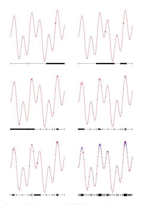
**Figure 4.3:** The first 5 iterations of the SOO algorithm and the resulting tree  $\mathcal{T}_n$  after n = 150 function evaluations. Here  $f(x) = (\sin(13x)\sin(27x) + 1)/2$  and K = 3. The blue dots represent the evaluations of the function at the center of the cells. The circle around the dots and the bold segments shows the nodes that are expanded at each iteration.
