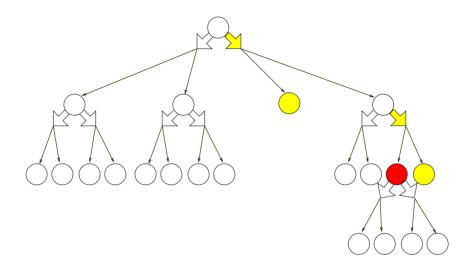
**Figure 5.3:** Among the leaves of the current optimistic subtree, the one with the largest contribution  $p(i)\frac{\gamma^{h(i)}}{1-\gamma}$  is expanded (represented in red): a call to the model returns the rewards and transition probabilities to the next states for each action.
