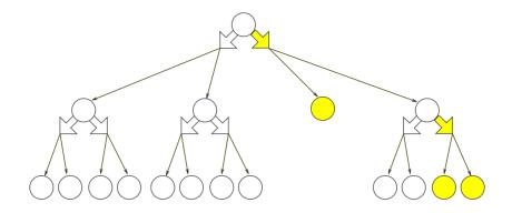
Figure 5.2: The subtree corresponding to the set of states that can be reached from the initial state. The big arrows represent the actions (K = 2) and the thin arrows the transitions to the next states (N = 2). Here 4 nodes have been expanded. The optimistic policy and the leaves of the resulting optimistic subtree are represented in yellow.
