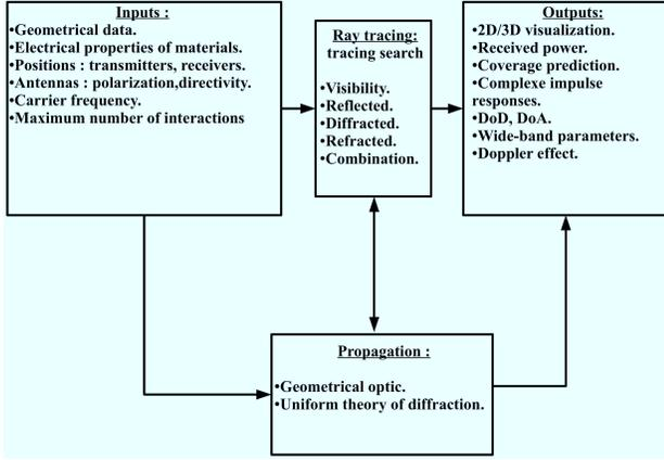
Fig. 1. Synoptic of the radio propagation simulator
