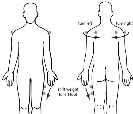
**Figure 3.** Two vibration motors were placed around each shoulder and laterally at the thigh that pointed forward during the ride. The arrows illustrate the direction of the stimuli on the skin. The labels describe the messages that the stimuli represented.
