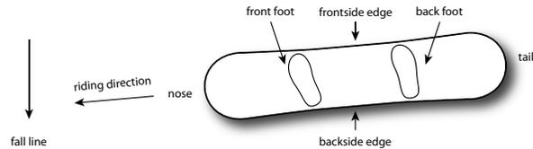
**Figure 2. Snowboard terminology and typical stance when the left foot points forward. Alternatively, some snowboarders prefer to descend with the right foot pointing forward. The fall line is the most direct path that a ball would roll down the hill.**
