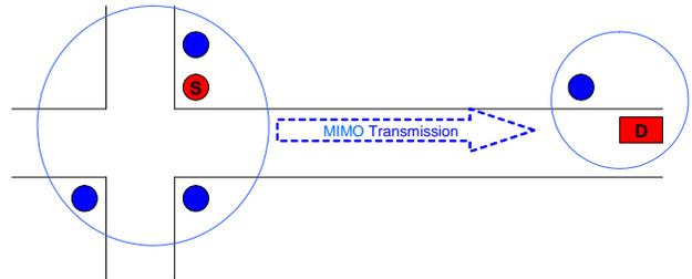
Fig. 9. Cooperative MIMO transmission between infrastructure and vehicle
