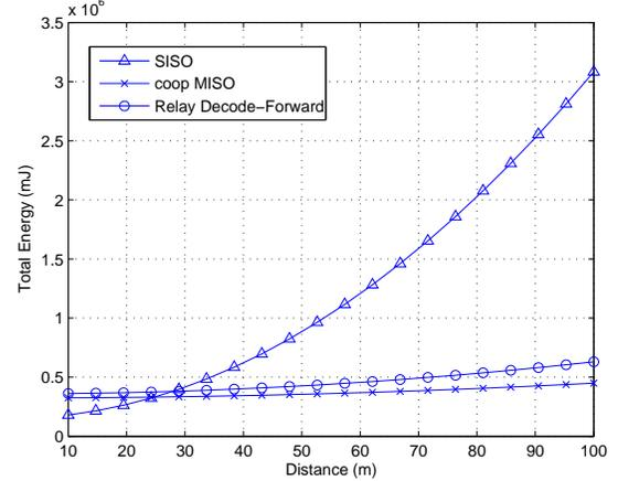
Fig. 18. Energy Consumption of relay technique vs. cooperative MIMO technique with two transmission nodes, error rate  $FER = 10^{-3}$ , power path-loss factor  $K = 2$ , source-relay distance  $d_1 = d/3$ .
