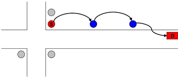
Fig. 6. Multi-hop SISO transmission between infrastructure and vehicle
