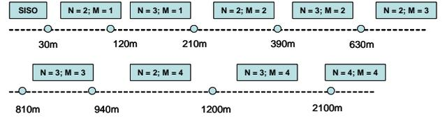
Fig. 17. Optimal  $N - M$  transmit and receive antennas set selection as a function of transmission distance,  $\Delta T_{syn} = 0.25T_s$ ,  $FER = 10^{-3}$  requirement, Rayleigh fading channel with power path-loss factor  $K = 2$ .
