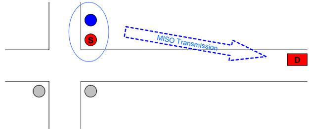
Fig. 8. Cooperative MISO transmission between infrastructure and vehicle
