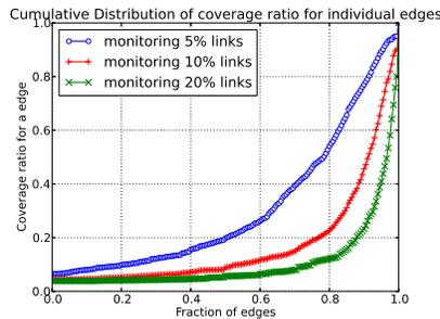
Fig. 4. Shortest path coverage ratio for individual edges
