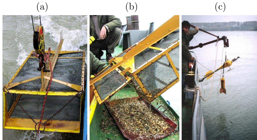
Fig. 2. Field measurements across the Danube section at km 1795.58: a) Basket-type bedload sampler (modified by VUVH); b) Bedload material collected from the sampler; c) Suspended-load sampler and torpedo current meter.
