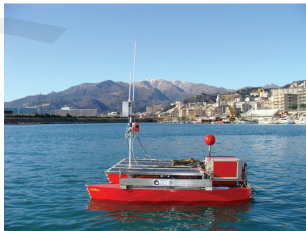
Figure 2. A view of the Charlie USV in the Genova Prà harbor. <AU: Please confirm that permission has been granted by the copyright owner to print this photo and please provide proper credit line.>
