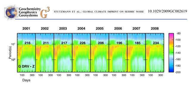
**Figure 4.** Seismic noise amplitude variations over 8 years in dB with respect to acceleration for the station DRV close to Antarctica. Bold numbers correspond to the number of days per year during which the primary microseism amplitude is below -150 dB (blue) in the period band 10-20 s.
