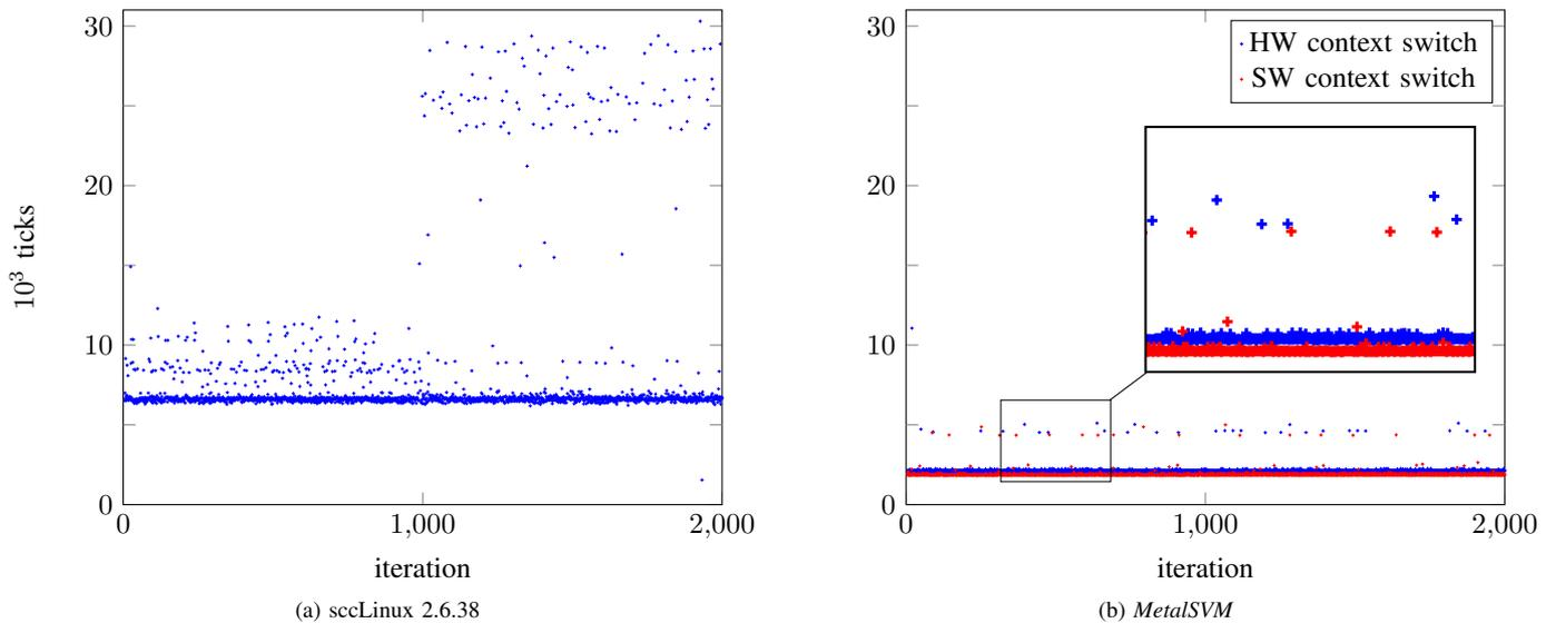
Fig. 3: Context switch latencies on the SCC (2000 iterations)
