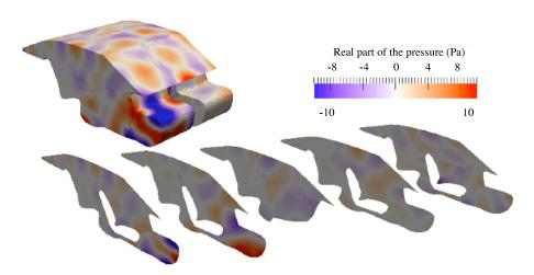
Figure 13. Real part of the pressure field computed with the 3-D VTRC in the problem defined in Figure 12 at 700 Hz.
