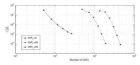
Figure 10. Scattering by a sound-hard sphere (Section 4.2): convergence curves for the relative solution error  $\varepsilon[p]$  (see (33)).
