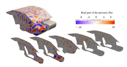
Figure 14. Real part of the pressure field computed with the 3-D VTRC in the problem defined in Figure 12 at 1200 Hz.
