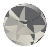
Figure 8. Scattering by a sound-hard sphere (Section 4.2): discretized computational domain.
