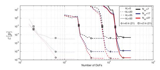
Figure 5. Cubic cavity (Section 4.1): convergence of the 3-D VTCR for the pressure field evaluation, with kL = 5, kL = 20, kL = 35 and kL = 50
