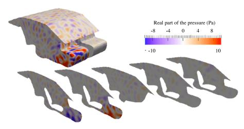
Figure 15. Real part of the pressure field computed with the 3-D VTRC in the problem defined in Figure 12 at 1700 Hz.
