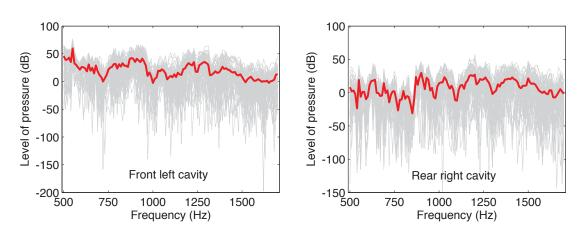
Figure 16. Evolution of the pressure of all the 64 points (grey curves) and the RMS average pressure (red bold line) inside the front left cavity (left) and rear right cavity (right) defined in Figure 12.
