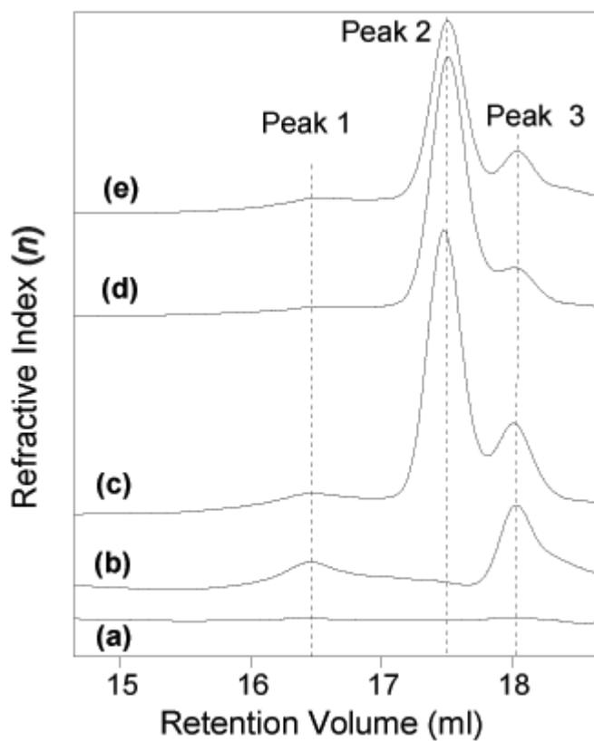
Figure 2. Gel permeation chromatography analyses of the raw migrates solutions. (a) Blank food simulant, (b) PLA-PF, (c) PLA-PF1, (d) PLA-PF2 and (e) PLA-PF3.
