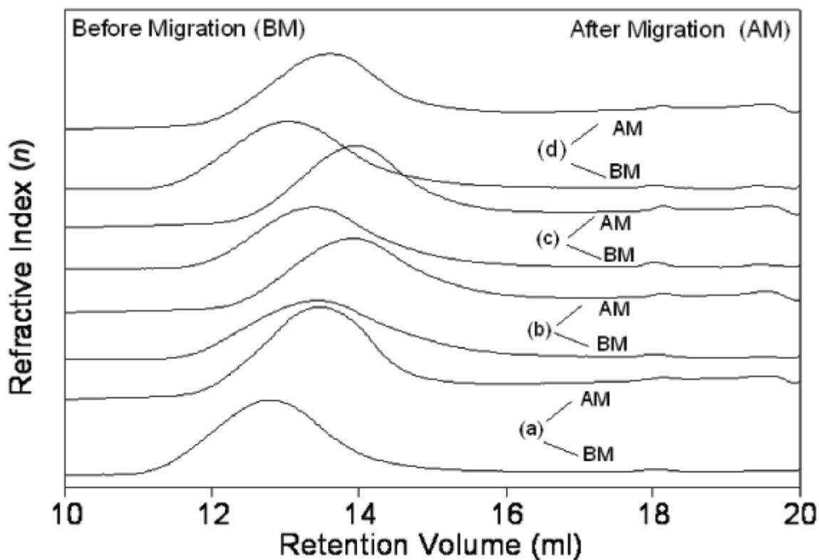
Figure 1. Gel permeation chromatograms of L-poly(lactide) (PLA) and PLA/laurate-modified Mg-Al layered double hydroxide (PLA-LDH-C<sub>12</sub>) films before (BM) and after (AM) migration experiments: (a) PLA-PF, (b) PLA-PF1, (c) PLA-PF2, (d) PLA-PF3.
