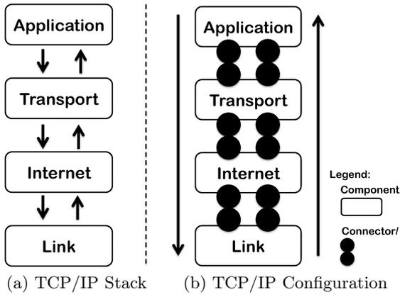
Figure 1: simplified version of the TCP/IP stack system.
