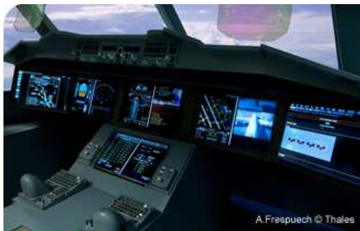
Figure 3: Example of HUD in an aircraft cockpit [4]
