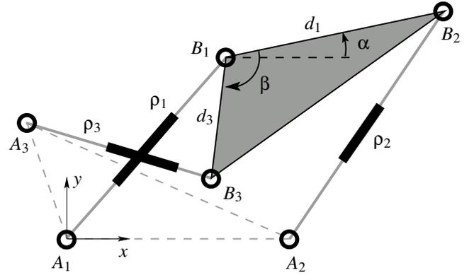
Fig. 1. Example of degenerate 3-RPR.
