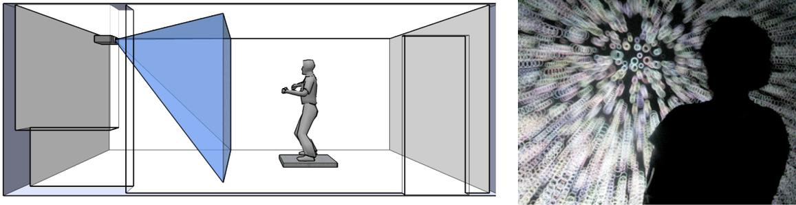
**Figure 1. Left:** Drawing of the *PIVViT* immersive platform, set up in an available room of the hospital. The large retro projected screen is at 60 cm of the patient, covering most of his visual field. The patient is standing on a force plate, recording center of pressure trajectories. **Right:** Photo of a patient viewing the forward-moving stimulus.
