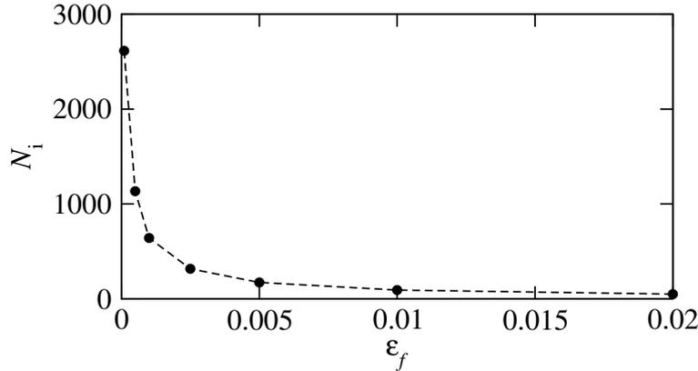
Fig. 10. The number of iterations  $N_i$  as a function of the precision criterion  $\epsilon_f$  in iterative resolution of the global SC problem when the forces are initialized to zero.
