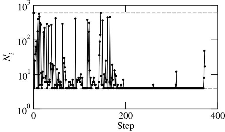
Fig. 11. The number of iterations  $N_i$  as a function of time step during a shear flow. The imposed minimum and maximum numbers of iterations are marked by dashed lines.
