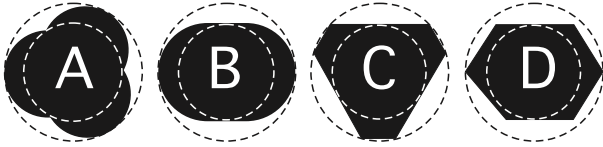
Fig. 2: Four different shapes belonging to the same \eta -set with \eta = 0.4 : trimer (A), rounded-cap rectangle (B), truncated triangle (C), and elongated hexagon (D).
