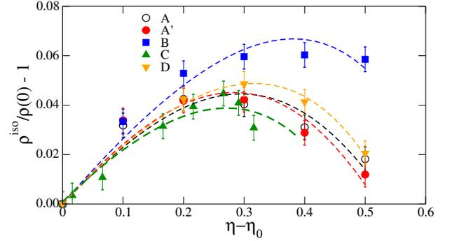
Fig. 8: Normalized packing fractions fitted by Eq. (6).
