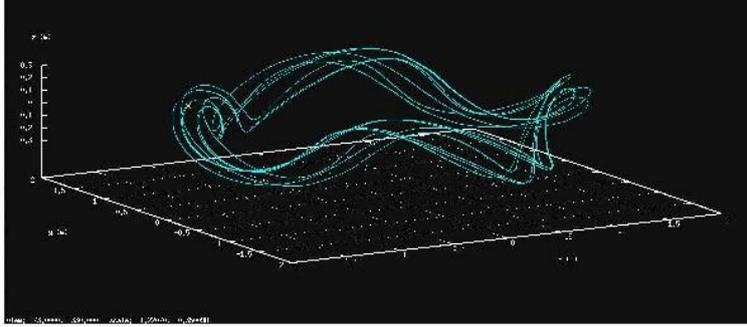
Figure 1. Particle trajectories in the TJ-II Stellarator
