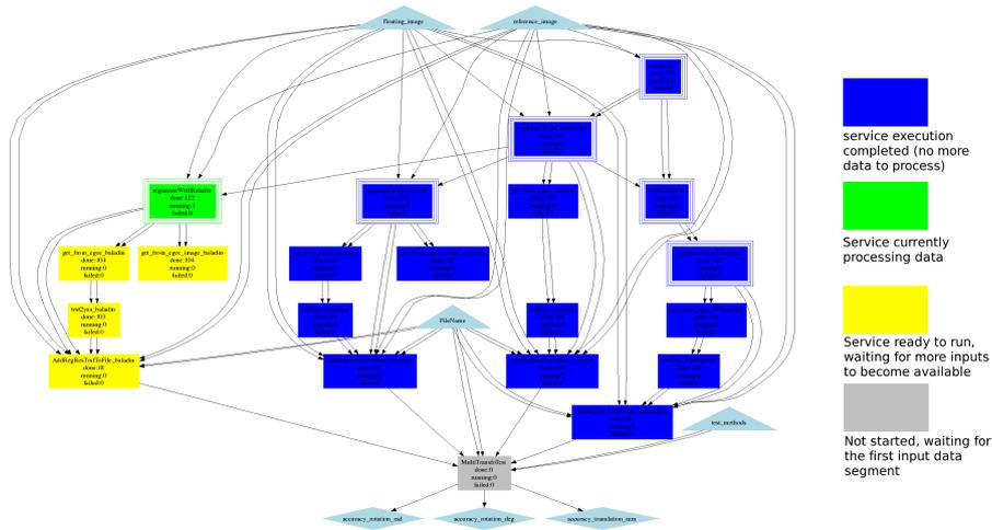
Figure 4. Bronze Standard application workflow: each box represents an image processing service and arrows show dependencies.
