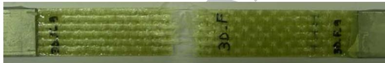
Figure 4. 3D composite loaded in fill direction, max stress 300 MPa: fatigue failure of a sample.
