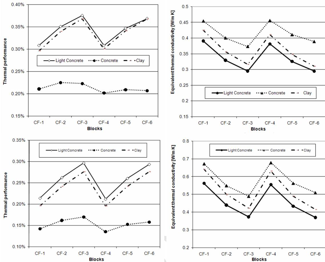
**Fig. 5.** Mass overall thermal efficiency (left) and equivalent thermal conductivity (right) for downward heat flow (upper) and upward heat flow (lower) for the three analyzed materials and six different models.
