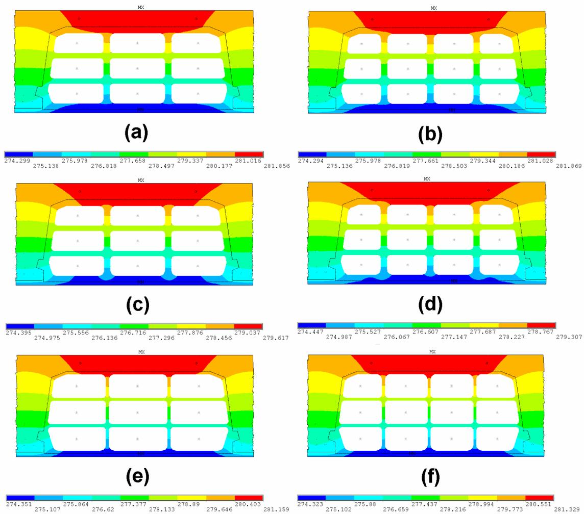
**Fig. 4.** Temperature distribution in floors made up of hollow block types *CF3* (left) and *CF6* (right) for the downward heat flow: lightweight concrete (a and b), normal concrete (c and d), and clay (e and f).
