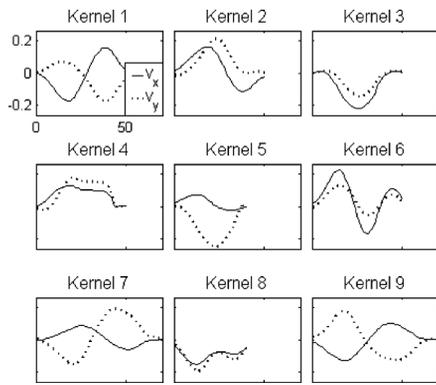
Fig. 2. Non-oriented learned dictionary (NOLD) of the velocities processed by 2DRI-DLA. Each kernel is composed of the real part  $v_x$  (solid line) and the imaginary part  $v_y$  (dotted line).
