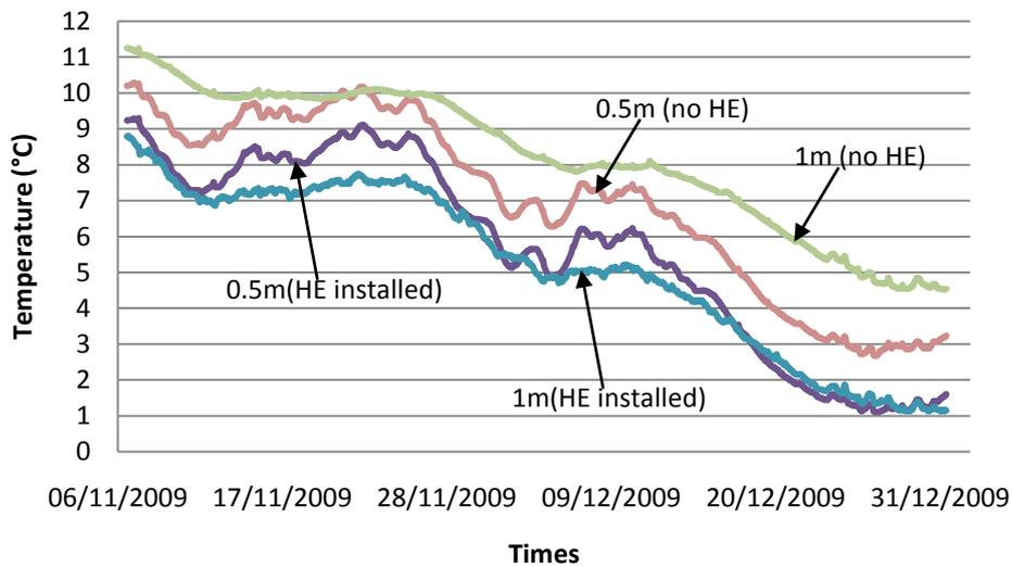
(c) At a depth of 0.5 and 1m below the ground surface
