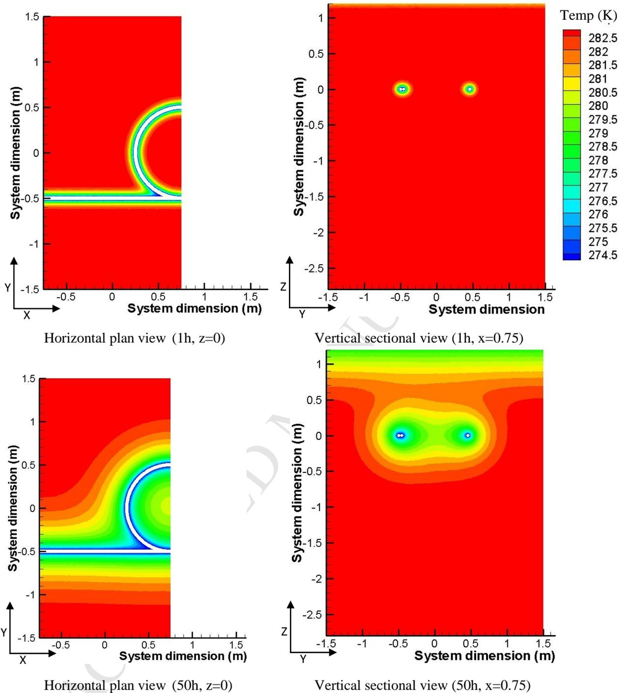
Figure 12 Isotherm generated from prediction for the slinky heat exchanger at 1 and 50 hours
