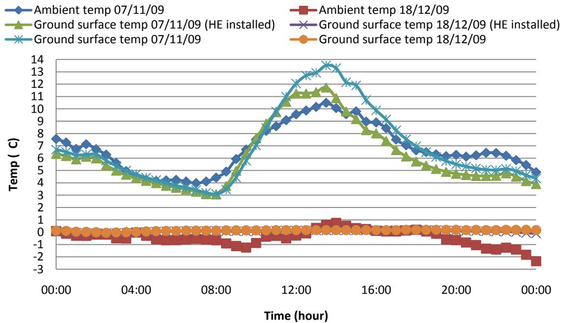
Figure 4 Measured ambient air temperature, ground surface temperature, solar radiation and wind speed on 7th Nov. and 28th Dec 2009
