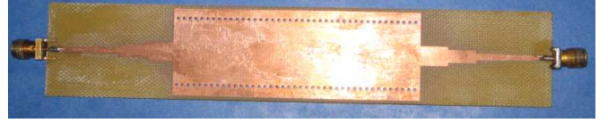
Fig.5. Photograph of the manufactured SIW with stepped transitions.
